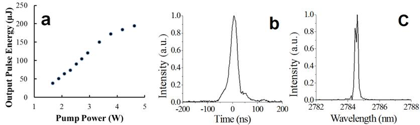
Fig. 8. Experiment result from Q-switched 3  $\mu\text{m}$  Er:ZBLAN fiber laser. (a) Pulse energy as a function of pump power at 1 kHz; (b) Output pulse train with a pulse energy of 201  $\mu\text{J}$ ; (c) A sample laser output spectrum.
