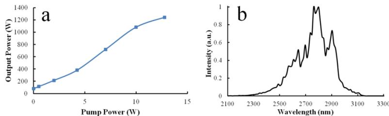
Fig. 2. OPA output. (a) output power as function of pump power; (b) Output spectrum.
