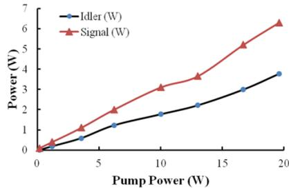
Fig. 4. OPA output power as function of pump power.
