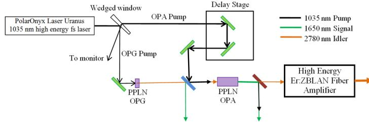
Fig. 1. Systematic diagram of 3  $\mu\text{m}$  seed and power amplifier system.
