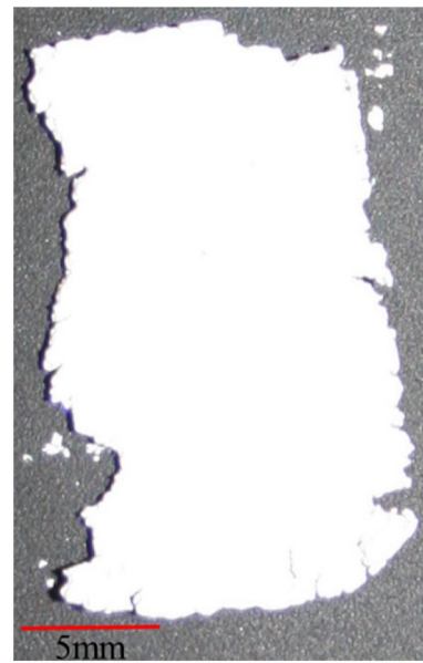
Fig. 8 Picture of good melting layer prepared under laser power of 131 W and scanning speed of 300 mm/s, hatching space of 30 \mu\text{m}
